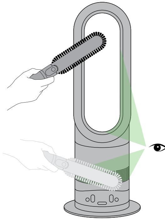
Ensure the heater is unplugged and has been allowed to cool.
