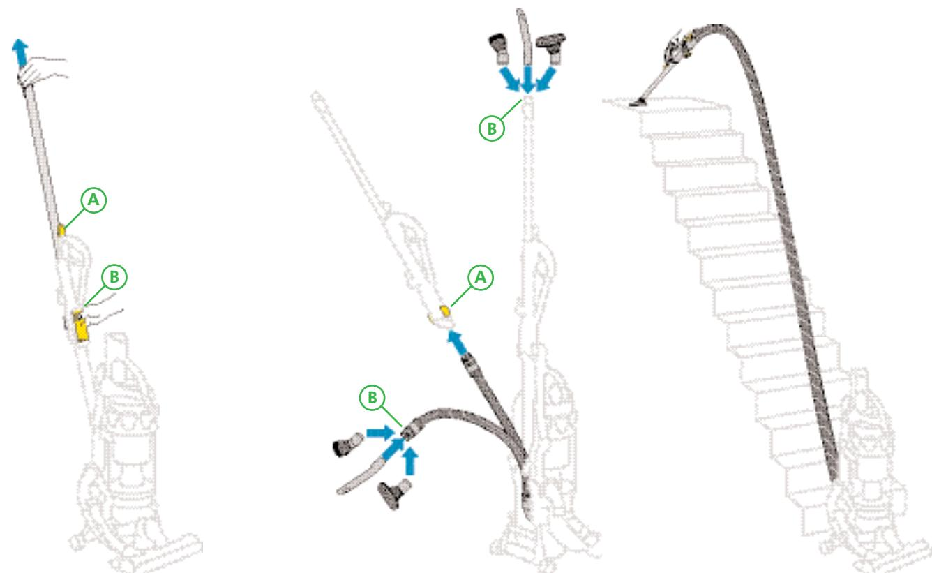
**UK** **Using the tools - Wand mode** **A** Pull metal wand from inside handle until it clicks. **B** Press button to release. When finished, ensure hose is straight then press button and push wand inside.
