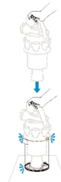
**UK** **Cleaning the shroud (optional)** - Empty bin and leave base open. Press catch **A** to detach clear bin.
